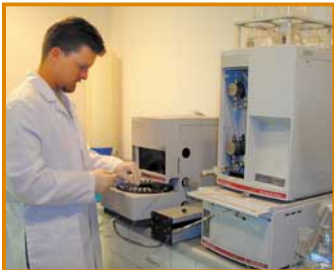
Here high-pressure liquid chromatography is being used for determining concentration.
