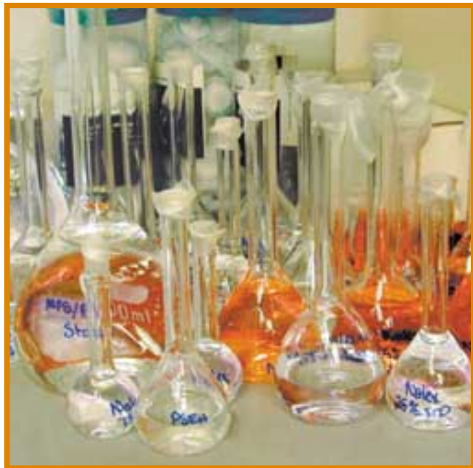
These volumetric flasks are used for preparing dilutions prior to analysis.
